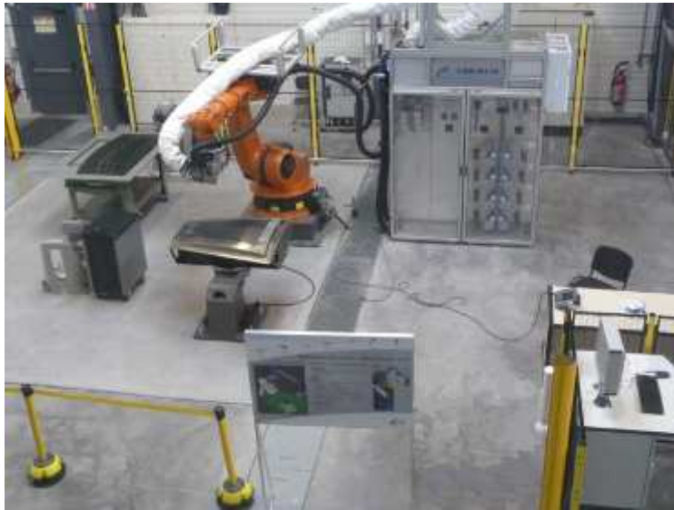
dry fibers placement
