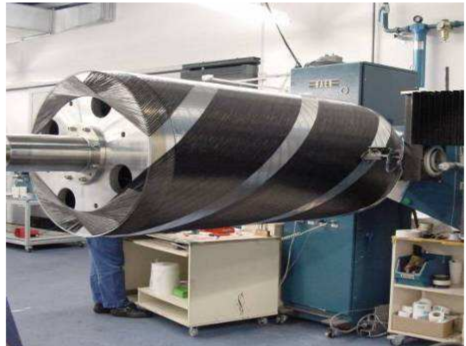
Filament Winding Telescope Cylinder
